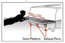
**Blockage of exhaust outlets** can cause carbon monoxide to accumulate in the cabin and cockpit area - even when hatches, windows, portholes, and doors are closed.
